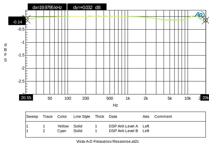
FIGURE 24. 96K/24BIT, MICROPHONE IN, FREQUENCY RESPONSE
