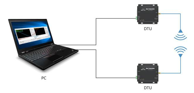
3. Firing up two XCOMs, choosing Baud rate 9600bps, 8N1, the setting which serial port transmission can be achieved.
