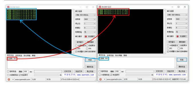
4、 User needs to open the mode switch first before link DTU with computer if the user want to modify parameters. Firing up <u>E34-DTU</u> 数传电台配置软件 (E34-DTU parameter configuration application) to modify related parameters. The mode switch must be reopened to achieve transmission after the configuration.
