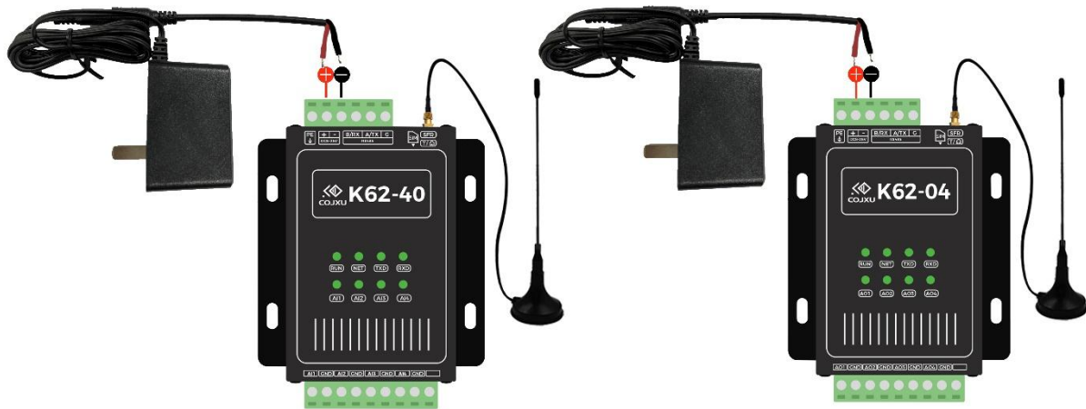
Figure 2-2 Product connection antenna and power supply
