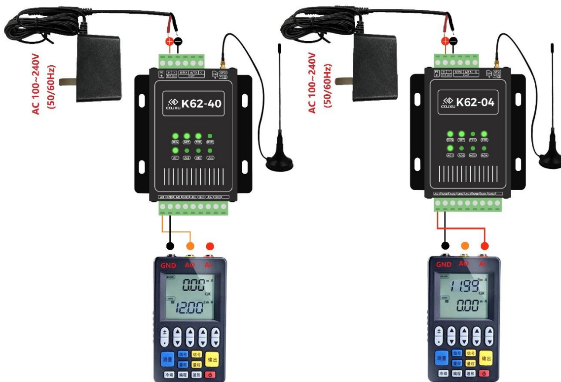
Figure 2-4 Observe the current value of the analog input and output modules
