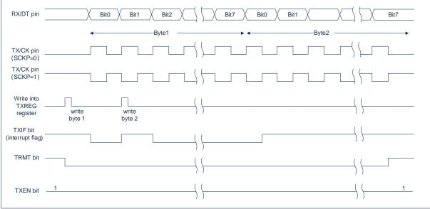
Fig 13-6: synchronous transmit
