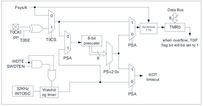
Figure 8-1: TimeR0/WDT module structure diagram
