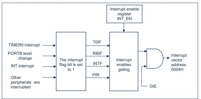
Figure 7-1: Schematic diagram of the interrupt principle
