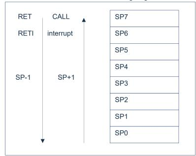
Figure 2-2: Stack memory processor works
