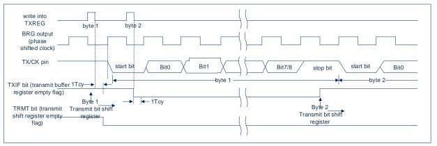
Fig13-4: asynchronous transmit (back to back)
