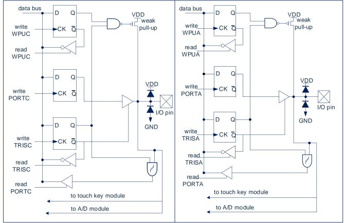
Fig. 6-1: I/O structure diagram (1).
