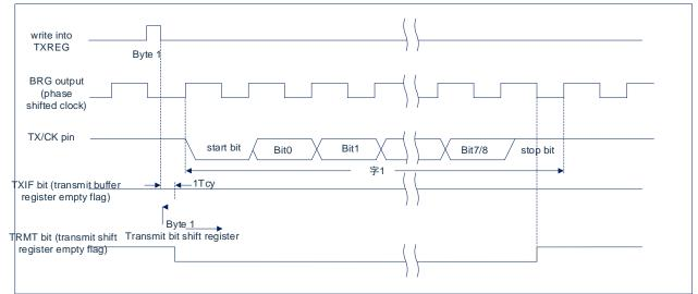
Fig 13-3: asynchronous transmit
