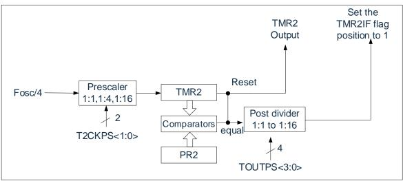
Figure 10-1: TIMER2 block diagram
