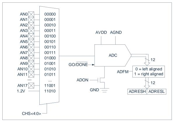
Figure 11-1: ADC block diagram
