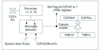
Figure 1 2-1: Capture mode working block diagram
