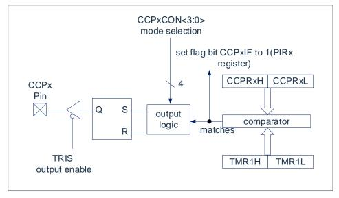
Figure 1 2-2: Compare mode working block diagram
