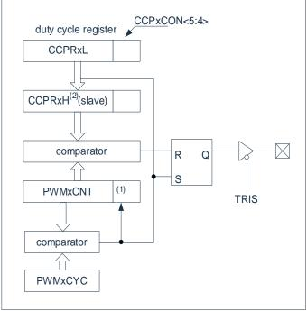
Figure 12-3: Simplified block diagram of PWM
