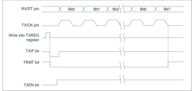
Fig 13-7: synchronous transmit (through TXEN)
