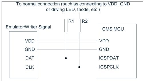
Figure 1-1: Typical online serial programming connection method
