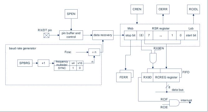
Figure 13-2: USART receive block diagram
