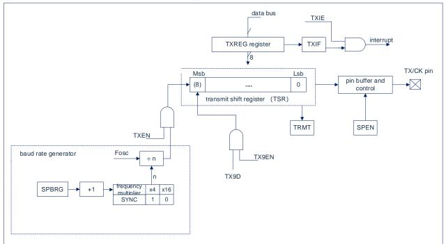
Figure 13-1: USART sends a block diagram
